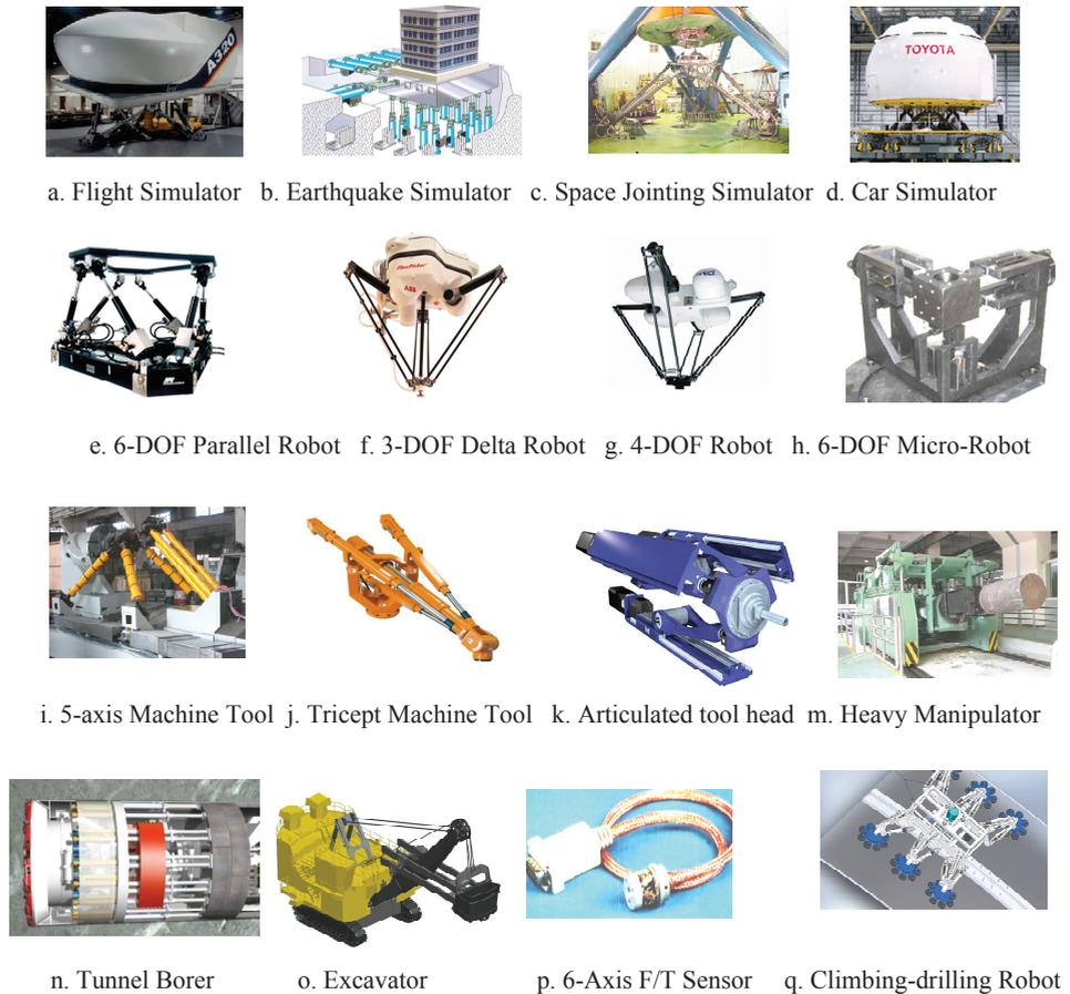
**Fig. 1.** Applications of parallel robotic mechanisms
