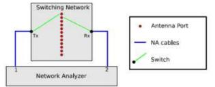
Fig.1. The switching network makes it possible to select one antenna for transmit and another for receive.
